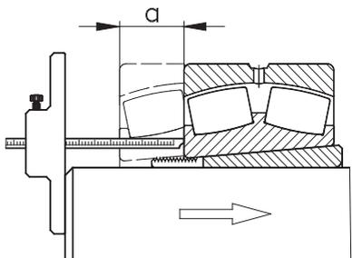
The actual distance of displacement "a" is measured using effective measuring instruments such as dial gauges, depth gauges or even simple calliper rulers. This may depend on the particular application.
